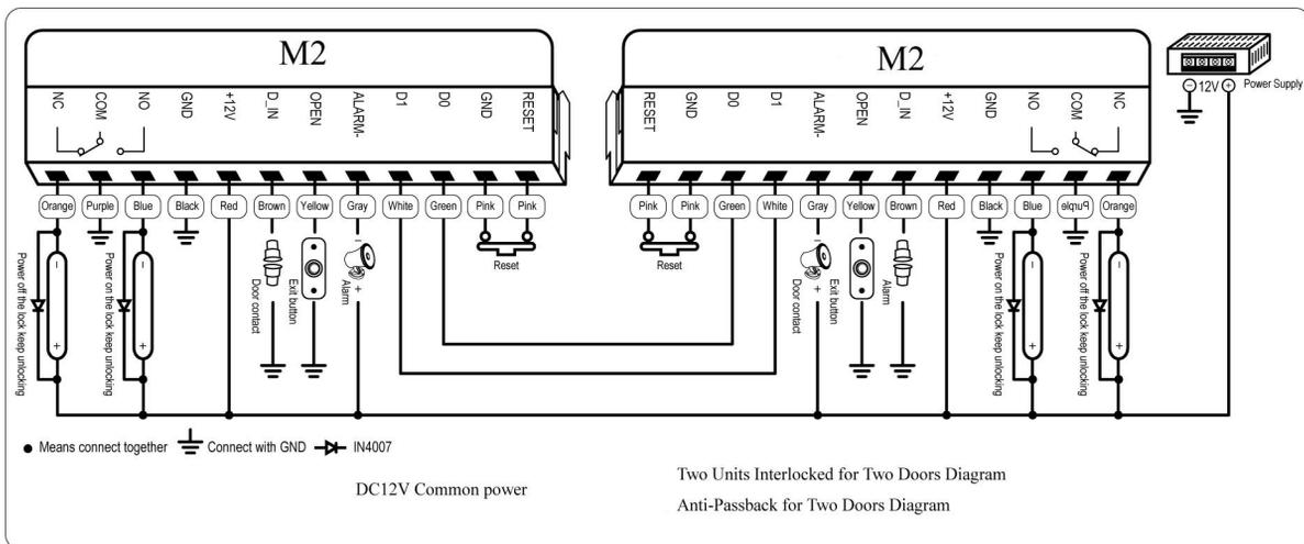
DC12V Common power Two Units Interlocked for Two Doors Diagram
